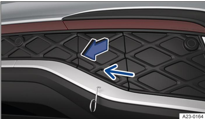
Fig. 3 In the rear bumper on the right: removing the cover.
