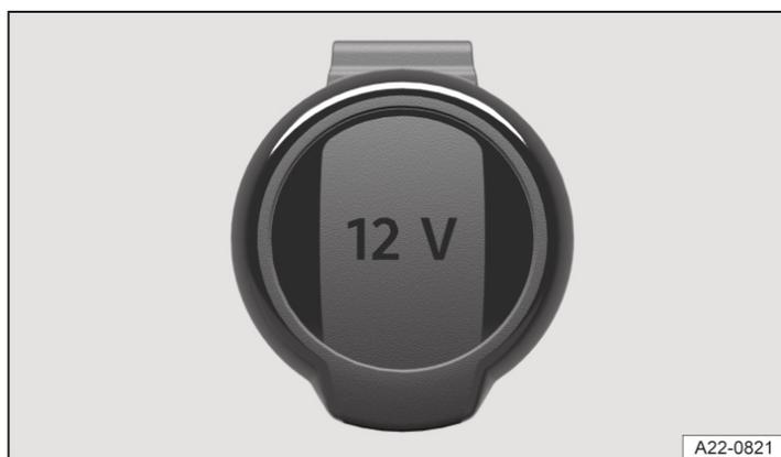
Fig. 1 In the stowage compartment in the centre console under the centre armrest, on the right-hand side of the luggage compartment: fold-open 12-volt socket (illustration).
