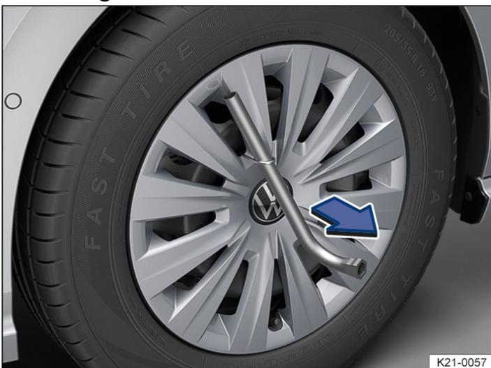
Fig. 1 Removing the wheel cover.
