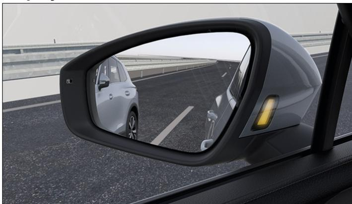
Fig. 1 In the exterior mirror housing: Side Assist displays.
