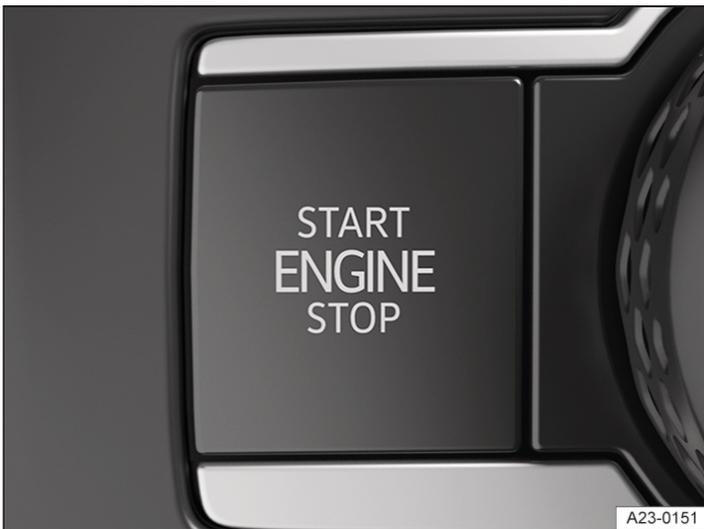
Fig. 1 In the lower section of the centre console: starter knob.
