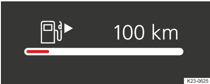
Fig. 1 In the digital instrument cluster: fuel gauge (illustration).
