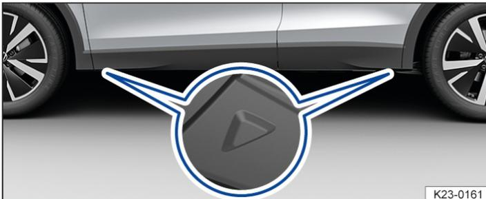
Fig. 1 On the sill: markings for the jacking points.
