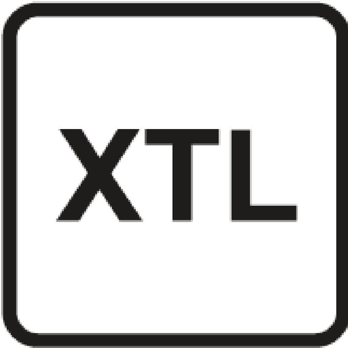
Fig. 6 Identification for synthetic diesel fuels.
