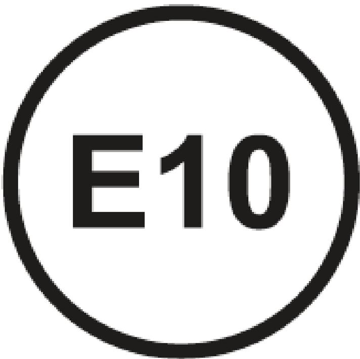
Fig. 3 Identification for petrol fuels with an ethanol content of 10 %.
