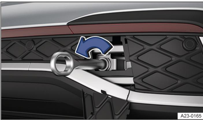
Fig. 4 In the rear bumper on the right: screwing in the towing eye.
