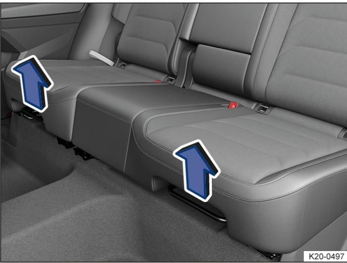
Fig. 1 Under the seat cushion of the rear bench seat: adjusting lever (illustration).
