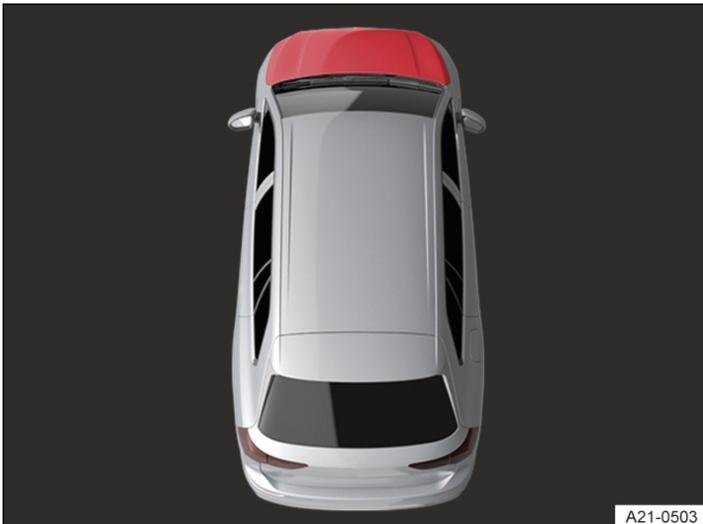
Fig. 3 On the instrument cluster display: the bonnet is open or not closed properly (illustration).
