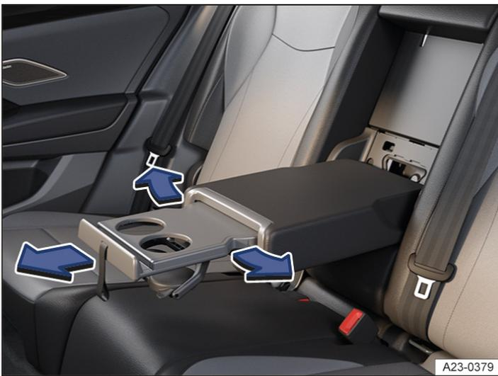
Fig. 2 In the rear centre armrest: pull-out stowage system (illustration).
