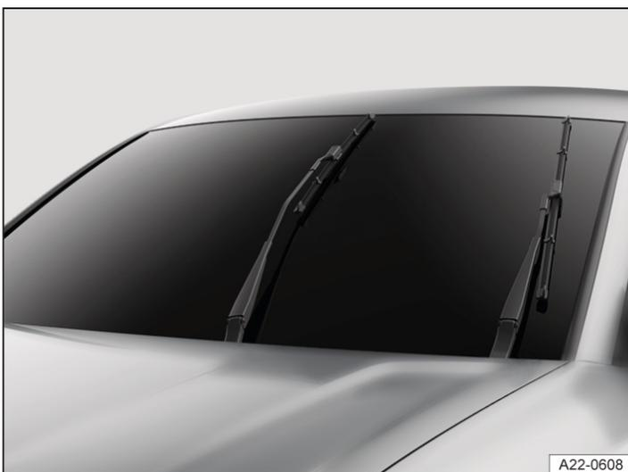
Fig. 1 Wipers in service position (illustration).
