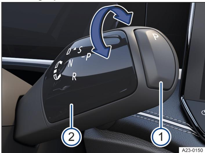
Fig. 1 On the right of the steering column: driving mode selector of the automatic gearbox.
