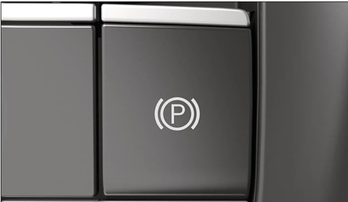
Fig. 1 In centre console: button for the electronic parking brake.
