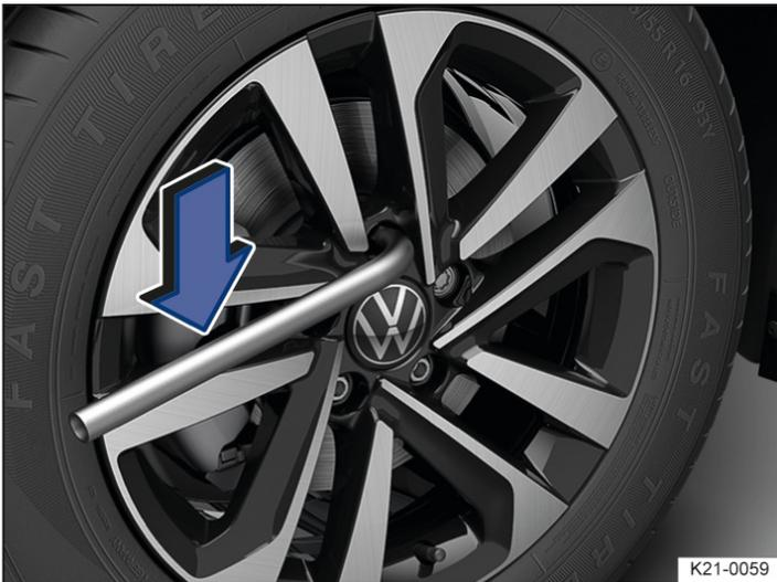
Fig. 1 Loosening wheel bolts.
