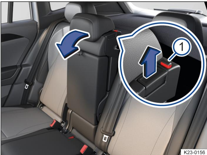
Fig. 3 Rear bench seat: folding the middle seat forward and back.
