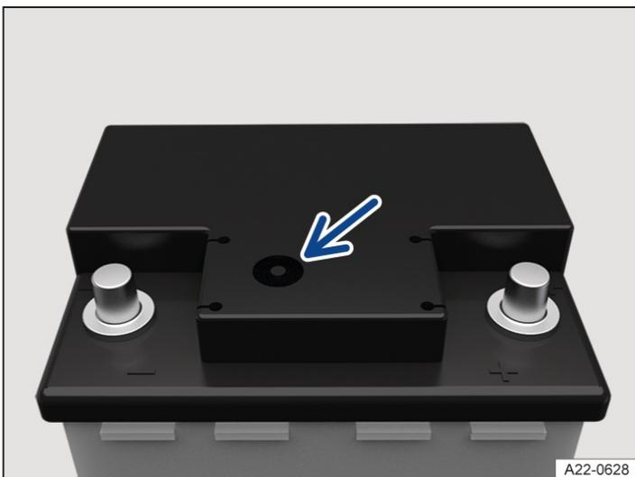
Fig. 1 On the top of the 12-volt vehicle battery: battery window (illustration).
