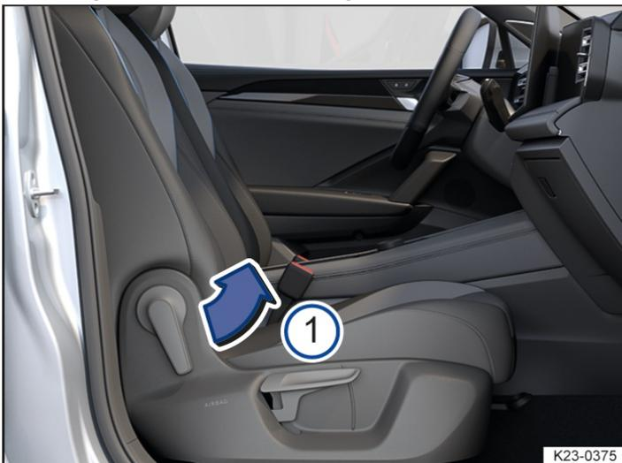
Fig. 1 Front passenger seat: folding backrest forwards.
