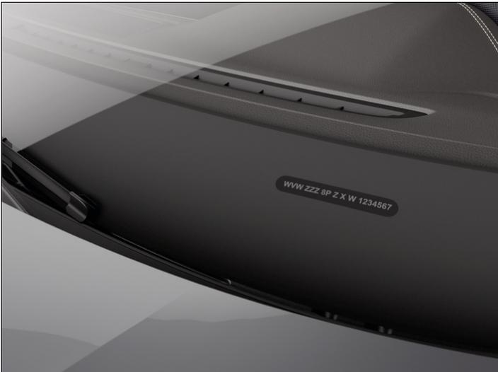
Fig. 1 In the windscreen: vehicle identification number.
