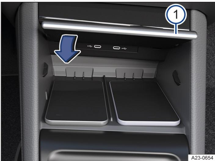
Fig. 2 In the centre console: stowage compartment with folding shelf (illustration).
