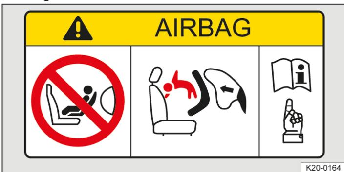
Fig. 1 On the sun visor: airbag label(illustration).
