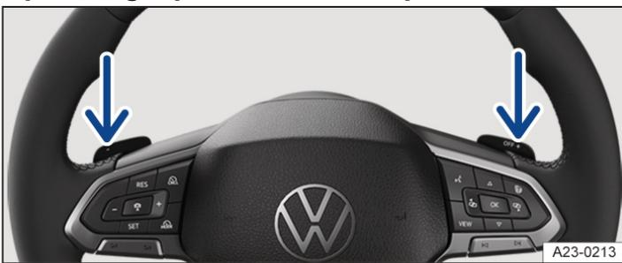
Fig. 1 Behind the steering wheel: paddles for Tiptronic.
