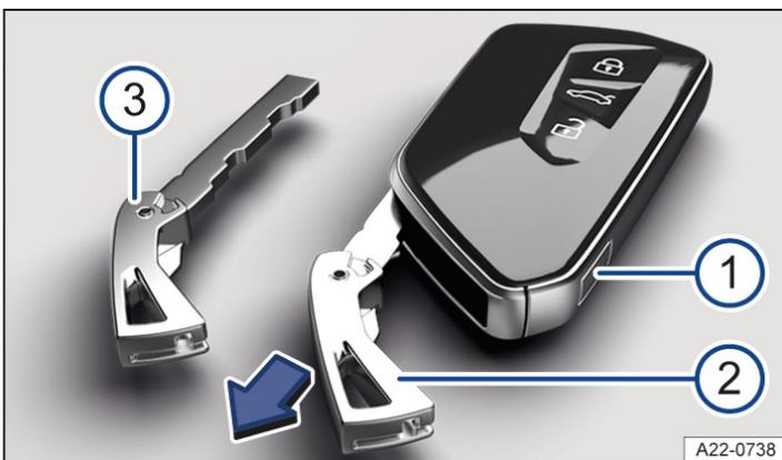
Fig. 1 Vehicle key: releasing the manual key.
