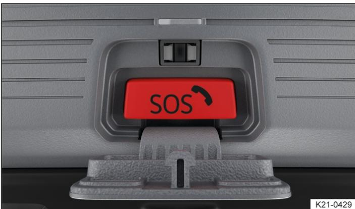
Fig. 2 In the roof console: button for Emergency Call Service.
