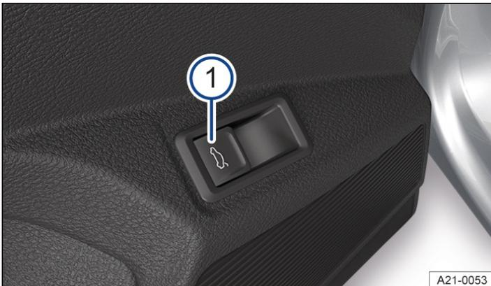
Fig. 2 In the driver door: button for opening or closing the boot lid electrically (illustration).
